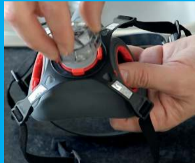
Remove exhalation valve cover
