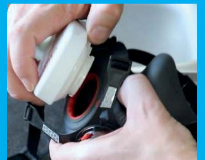
Replace filters (new pair if required).
